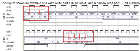
In this example, the read port is operating at twice the frequency of the write port. Writing two 16-bit words to the FIFO buffer increases the wrusedw flag to two and the rusedw flag to four. Four 8-bit read operations empty the FIFO buffer. The read begins with the least-significant 8 bits from the 16-bit word written followed by the most-significant 8 bits.
