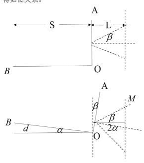
\(L、X、S\)已知,则\(tan2\alpha=\frac XL\),\(2\alpha \to 0\)\\(\alpha = \frac X{2L}\),so\(d=S tan\alpha=s\alpha=\cfrac{XS}{2L}\).
